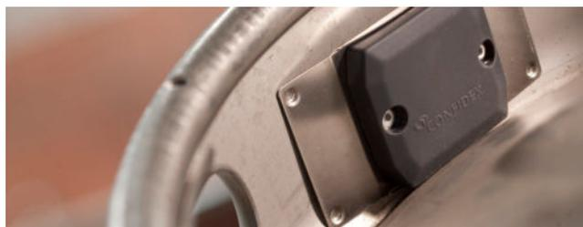
When the application is too demanding for adhesives, but the metal surface cannot be punched for screw or rivet fixing, welding the tag with special bracket is an option for attachment. Welding bracket is made of stainless steel and delivered ready attached to tag with pop rivets. Bracket design allows attachment on both flat and curved surfaces.
